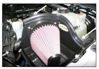
**8.** Install the Airaid Premium Filter (#1) onto the adapter tube and tighten the hose clamp. Next install the weather strip (#5) onto the top of the Quick Fit panels as shown
