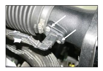
7. Reinstall the MAF sensor into the Airaid Adapter Tube using two 8-32 x 3/8" button head screws (#11). **Do Not Use The Factory Screws!**
