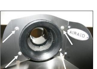
**5.** Install the **MAF** Adapter Tube (#2) into the Quick Fit Panel as shown using four 1/4-20 button head bolts (#9) and flat washers (#10). Make sure the slot for the **MAF** sensor is on the left side when looking from this view.
