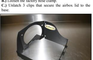
**4.** Assemble the two Quick Fit panels (#3 & #4) as shown using four 6-32 screws (#6) flat washers (#7) and kep nuts (#8). Apply the Airaid Decal onto the Panel assembly as shown.
