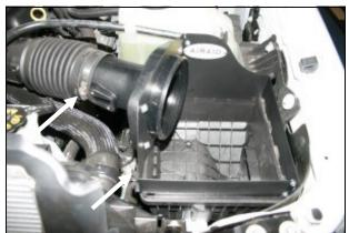
**6.** Install the Quick Fit Assembly onto the top of the factory airbox base sliding the four tabs on the panel into the slots on the base and then latching the three factory latches. Slide the factory intake tube over the **MAF** tube and tighten the factory hose clamp as shown.
